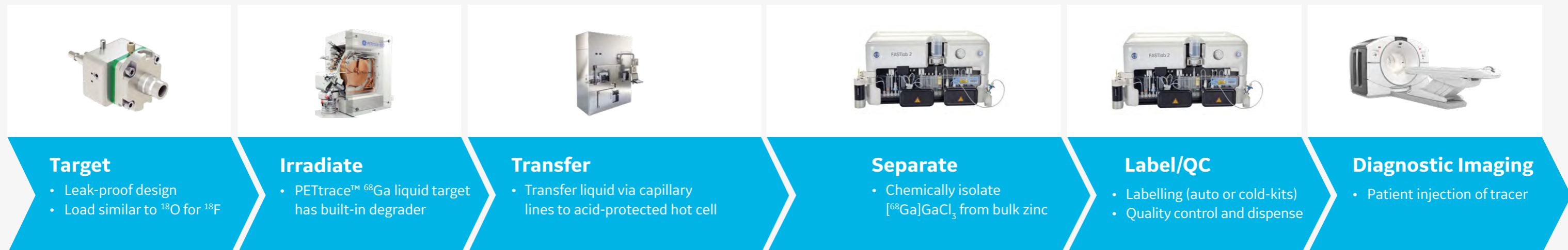
Figure 2 – High level workflow for cyclotron production. Images may not be representative.
