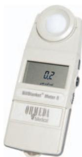
**BiliBlanket Light Meter II** – Provides a reliable measure of light emission performance from phototherapy systems.
